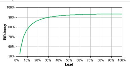
Curve fit to measured efficiency data. All measurements taken in normal operating mode, at typical environmental conditions, with nominal electrical input and resistive load output.
